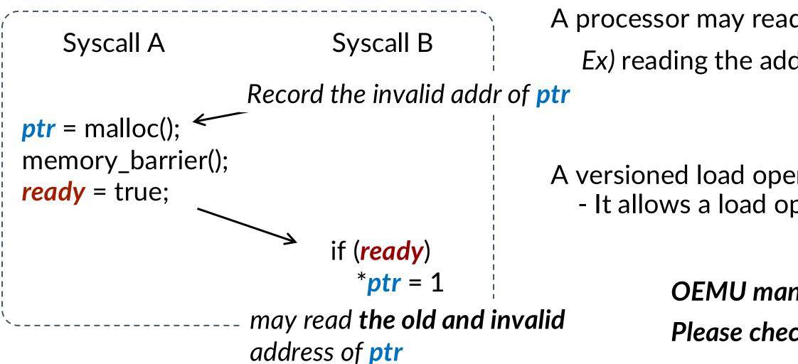
A processor may read memory *ahead* of *previous* instructions *Ex*) reading the address of *ptr* before *ready* in Syscall B
