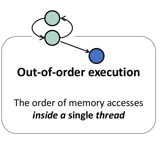
Controlling thread interleaving obscures the effect of out-of-order execution
