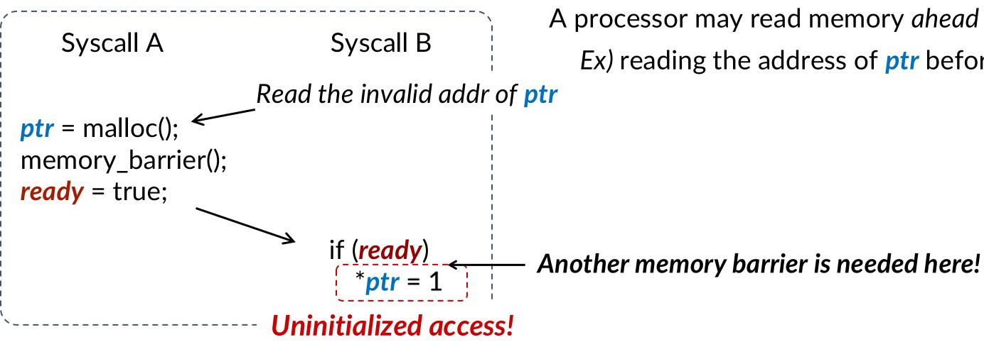
A processor may read memory ahead of previous instructions *Ex*) reading the address of *ptr* before *ready* in Syscall B
